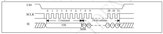
Figure 10-27a Block Erase 32K(BE32K) Sequence (QPI)
