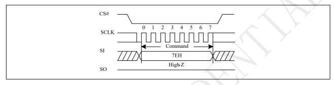
Figure 10-48a Global Block Lock (QPI)
