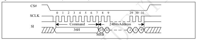
Figure 10-45a Individual Block Lock (QPI)
