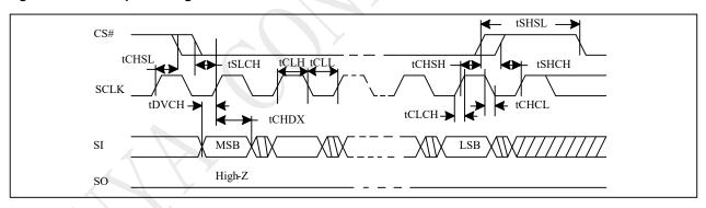
Figure 5-5 Output Timing
