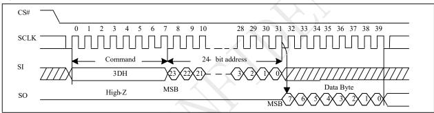
Figure 10-47a Read Block Lock Status (QPI)
