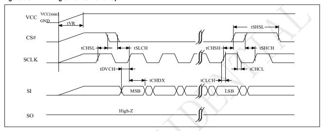
Figure 5-9 Power-Up Timing
