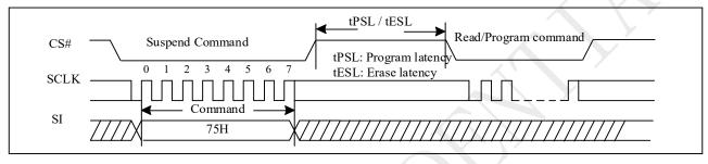
Figure 10-42a Suspend to Read/Program Latency (QPI)
