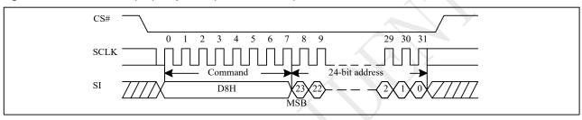
Figure 10-28a Block Erase (BE) Sequence (QPI)
