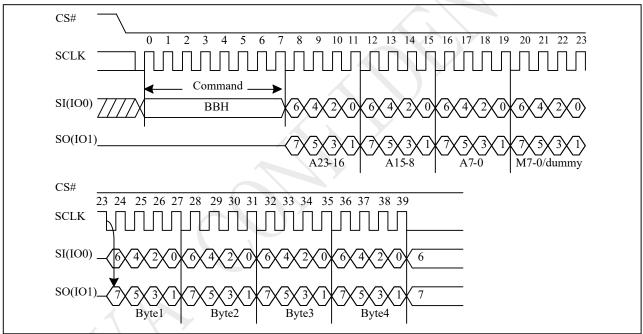
Figure 10-13 2IO Read Sequence (Command BBh M5-4 ≠ (1,0))
