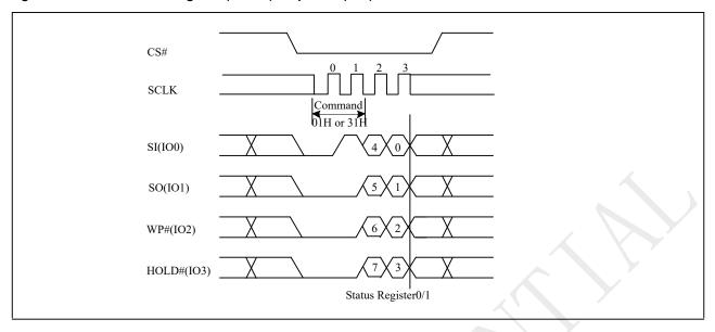
Figure 10-7b Write Status Register (WRSR) Sequence (Command 01, 2 bytes' data)
