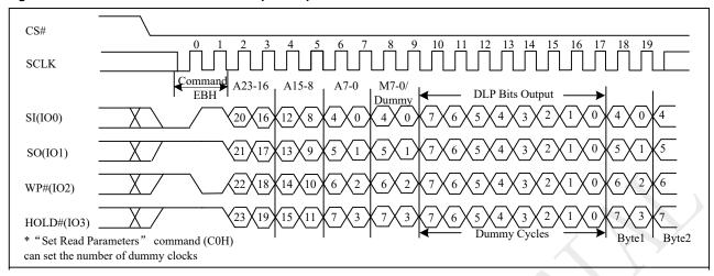
Figure 10-23h Burst Read with Wrap with DLP bits output Sequence
