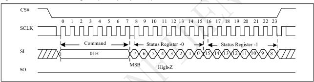
Figure 10-7c Write Status Register (WRSR) Sequence (QPI)
