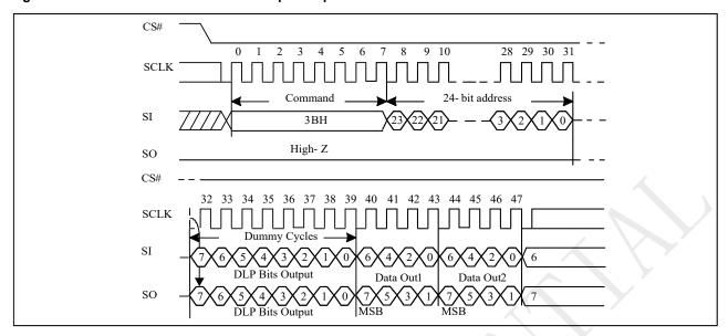
Figure 10-23c 2IO Read with DLP bits output Sequence
