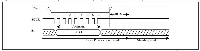
Figure 10-36c Release from Deep Power-down (RDP) Sequence (QPI)
