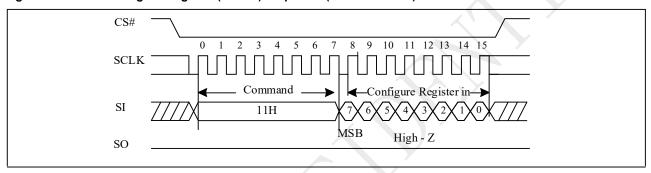
Figure 10-8a Write Configure Register (WRCR) Sequence (QPI)
