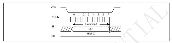
Figure 10-2a Write Enable (WREN) Sequence (QPI)
