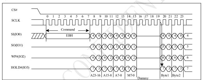
Figure 10-16 4IO Read Sequence (Command EBh M5-4 ≠ (1,0))
