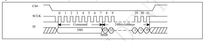
Figure 10-46a Individual Block Unlock (QPI)
