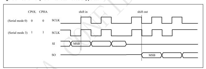
Figure 8-1 Serial Peripheral Interface Modes Supported
